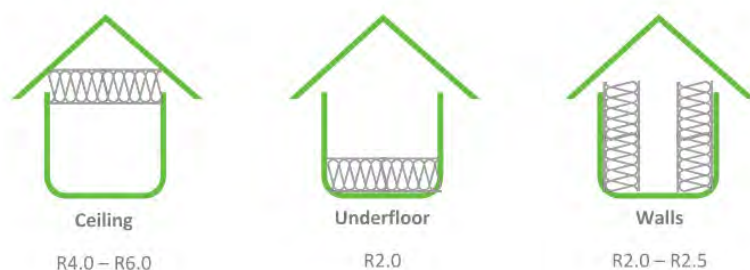
FIGURE 10 Recommended insulation R-Values per building element
